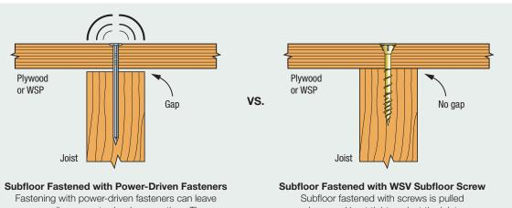
gaps or allow gaps to develop over time. These gaps cause the subfloor to ride up and down on the pneumatic fastener's shank, which leads to squeaks.
