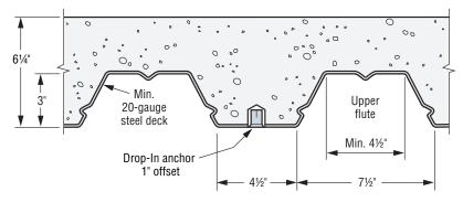
Figure 1. Lightweight Concrete over Steel Deck
