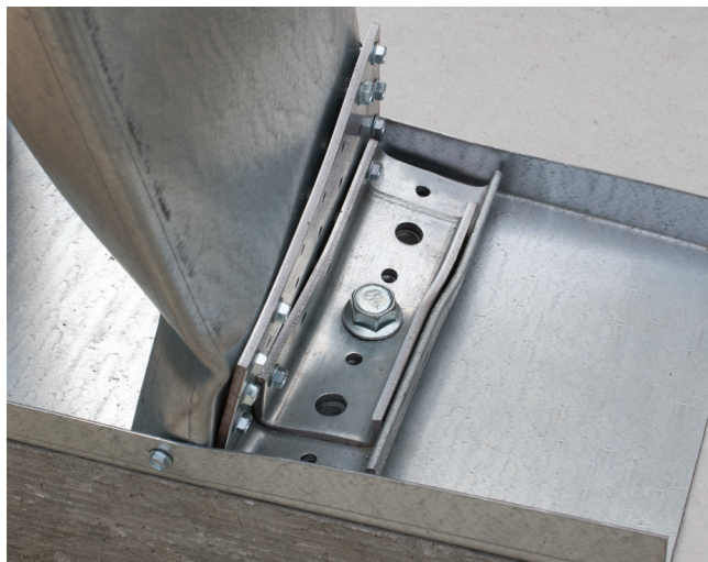
RCKW assembly test with member failure.
