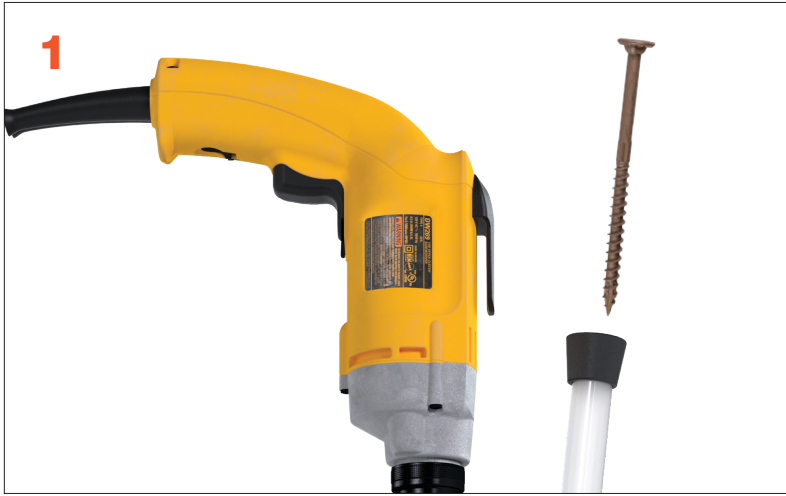
Drop a single structural screw into the feed tube.
