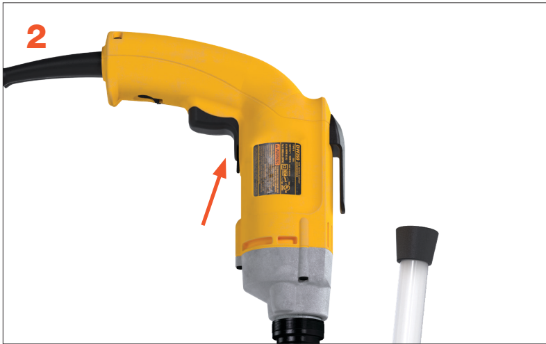
Pull the driver motor trigger.
